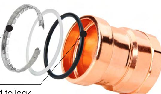
**Engineered sealing elements** are designed to leak before they are pressed, giving a visual indication of a connection that has not been pressed
